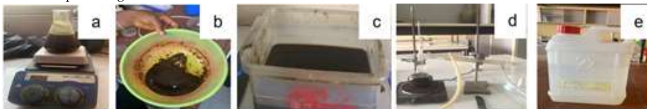
Figure 3: (a) mixture of B. vulgaris bamboo culm flour + sodium hydroxide (NaOH) solution; (b) B. vulgaris residue of enzymatic hydrolysis; (c) Mash – the fermented liquid - containing ethanol from bamboo flour; prepared/stored in a container
